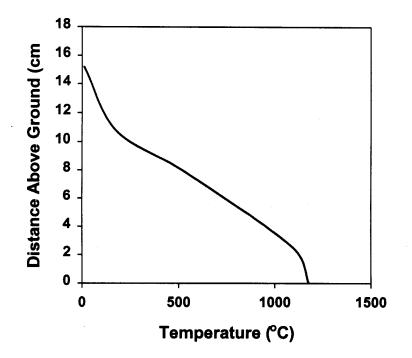
Fig. 2. Effect of distance from burner on the temperature experienced by the plant. Source Thomas, 1964
